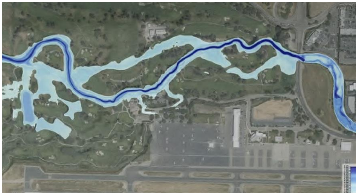
Figure 10: Inundation with Ten-Year Flow, 6-ft Wide Channel Grading (2:1 SS)
